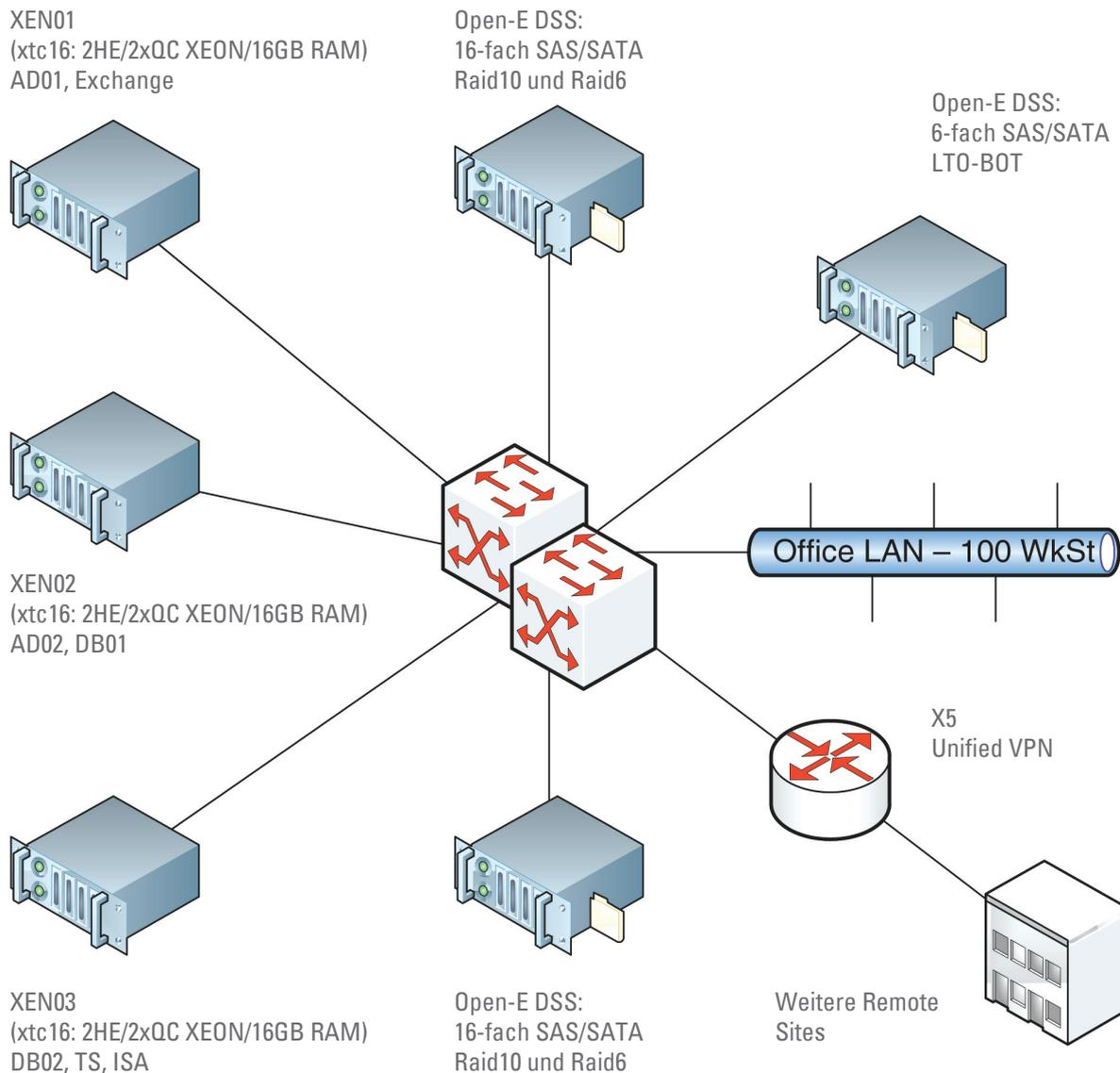
Virtualized infrastructure: following project planning and implementation, the company's IT is now housed in an optimized, efficient structure – scalable to a pronounced degree and providing maximum availability.
